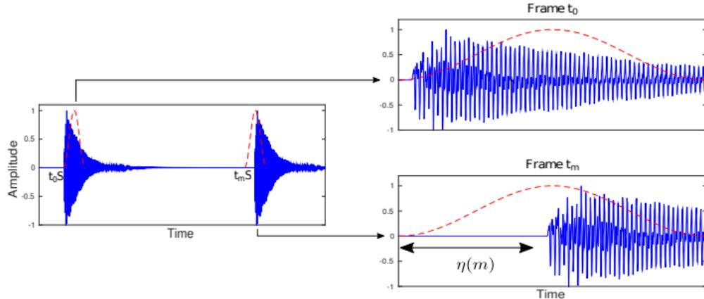
$$X(f, t_m) \approx X(f, t_0) \rho(m) e^{i\lambda(m)f}, \text{ with } \lambda(m) = \frac{2\pi\eta(m)}{F}.$$
